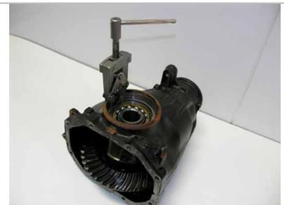
**Caution!** do not mix up bearing races and circlips. The preload of the pinion bearings, the backlash and tooth contact pattern will **not** have to be adjusted again provided the circlips and bearing races are reinstalled in their original positions, and the pinion assembly is not disassembled or altered in any way.
