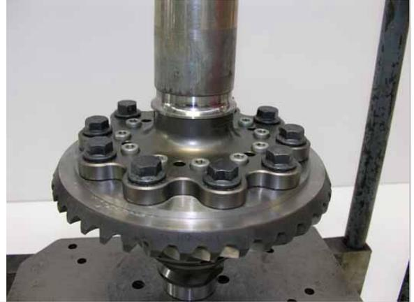
Install LSD gear set into the casing, lubricate bearings with gear oil. Install the left outer race and install the circlip. Press the Quaife gently from the right hand side to ensure the circlip is in the seated position. Install the right outer race and circlip. It may be necessary to press or tap in the right circlip, as this preloads the output bearings.
