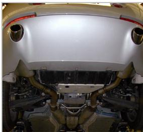
**Sport Rear Silencers** are not part of the engine conversion, but manufactured in lightweight stainless steel, they improve the aural quality of the exhaust, and whilst they still meet the criteria of the European D4 noise limits, the tonal change improves the sound to a deep rumble.
