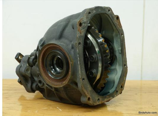
2. Clean out any residual oil from inside the housing.
