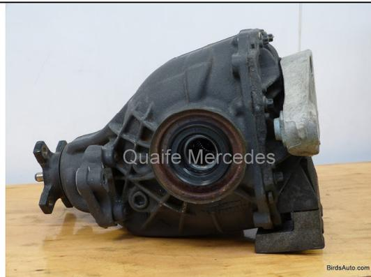
Final drive unit from a 216 CL 65 AMG. The final drive is already removed from the vehicle paying attention to the manufacturers instructions. Damage may occur if you do not work in accordance with manufacturer recommendations.
