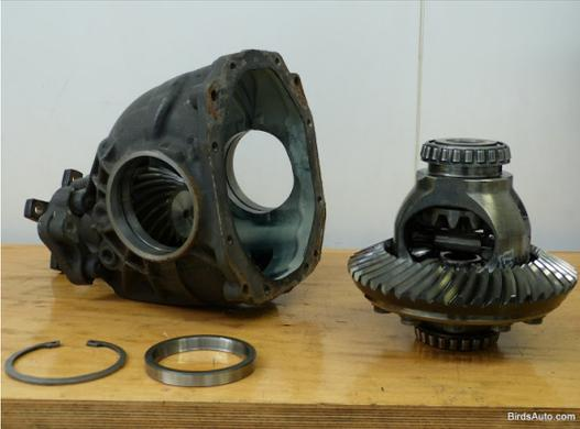
5. Remove bearing outer race retainers.
