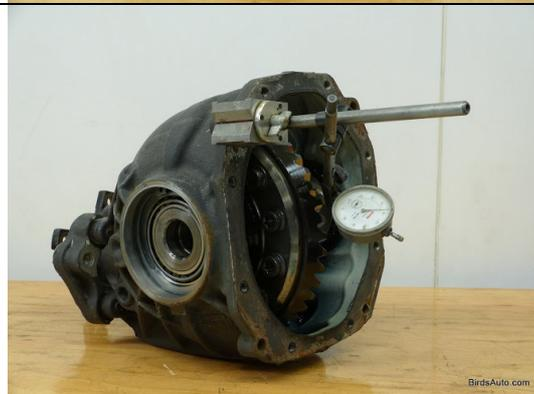
4. Check and record the crownwheel to pinion backlash. Typical backlash figures are between 0.06 and 0.14mm, and largely depend on the size of the crownwheel.
