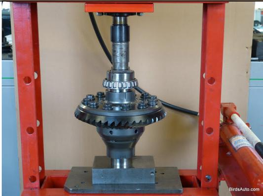
15. Press on the bearing inner races on the correct sides, taking care to ensure the races are fully bottomed out on the Quaife bearing journal.
