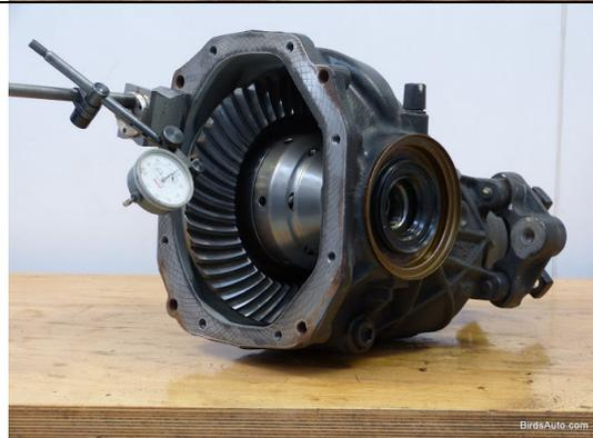
19. Check the crownwheel to pinion backlash. It is common to note that the backlash has decreased slightly from original. This is due to the fact that the final drive has not yet been run.
