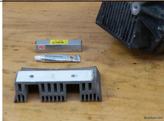
In this case, the standard differential cooler has to be removed. Clean off aluminium oxide, and apply heat sink compound, which improves the effect of the cooler.
