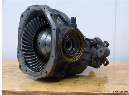
18. Install new output shaft seals.
