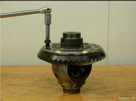
9. Remove the standard bolts from the crownwheel, and remove the crownwheel by tapping with a drift.
