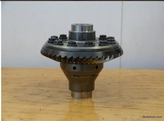
14. Add Loctite or Wurth ThreadLock Medium strength to the original bolts and torque to the factory settings.
